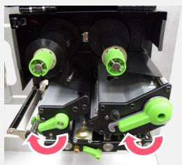
3. Thread the leading edge of the label through the media guide bar pass media sensor, and place the leading edge onto the platen roller.
