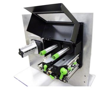
2. Open print head release lever and label guide bar release lever to thread the label through the front of the print engine and remove several labels.
