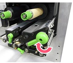
4. Thread ribbon above the ribbon guide bar and through ribbon sensor slot.
