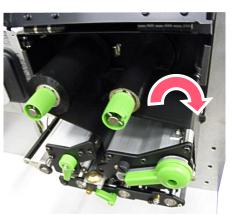
6. Close the print head mechanism by pushing the print head release lever.
