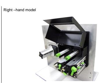
2. Install the ribbon and paper core onto ribbon supply spindle and ribbon rewind spindle.
