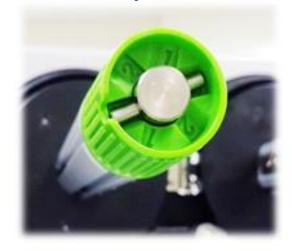
**Ribbon Supply Spindle Tension # 3**
