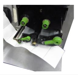
4. Adjust the rear label guide to fit the label width.
