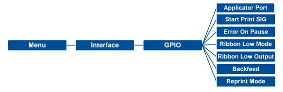
**Default Description Item** This option is used to set the GPO\_3 signal when PRINT END. Selections Description The applicator port is off. Off Label Label Waiting Label prints Ready for next format format for start processed print label sent signal Not ready Data ready Ready Off **Applicator Port** (Pin 14, GPO\_6) Mode 1 Do not start Print start Start (Pin 3, GPI\_1) Do not end Print End End (Pin 11, GPO\_3)
