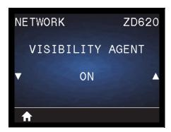
**Description:** When the printer is connected to a wired or wireless network, it will attempt to connect to Zebra's Asset Visibility Service via the Cloud-based Zebra Printer Connector using an encrypted, certificate-authenticated web socket connection. The printer sends Discovery Data and Settings and Alerts Data. Data printed via any label formats is NOT transmitted.
