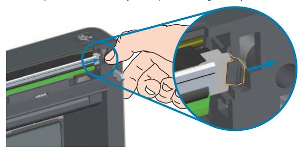
3. Swing the loose right side of the printhead out of the printer. Pull it out and to the right a little to get the left side of the printhead clear. Pull the printhead out and free of the top cover to gain access to its attached cables on the backside of the printhead. Note, the red highlights the left side printhead retainer slot.
