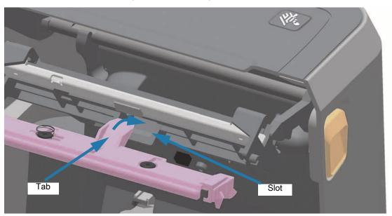
**4.** Insert the left side tab of the printhead assembly into the recessed slot on the left side of the Printhead Actuator Arm.
