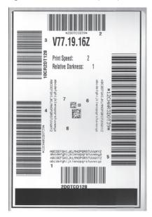
**4.** See Figure 3 and Table 2. Inspect the test labels and determine which one has the best print quality for your application. If you have a barcode verifier, use it to measure bars/spaces and calculate the print contrast. If you do not have a barcode verifier, use your eyes or the system scanner to choose the optimal darkness setting based on the labels printed in this self test.
