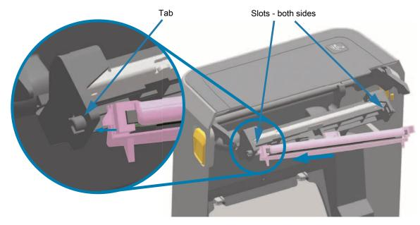
**5.** Push the right side of the printhead into the printer until the latch locks the right side of the printhead into the printer.
