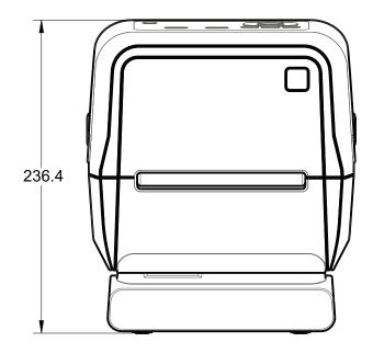
Printer with Attached Power Supply Base
