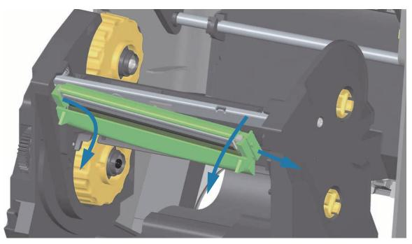
**4.** Gently but firmly pull the two printhead cable bundle connectors off of the printhead.
