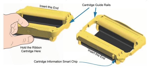
1. Insert the ribbon cartridge into the ribbon cartridge slot on the ribbon transport in your open printer. Push until the cartridge is nearly flush to the front of the ribbon transport. You will hear and feel the cartridge lock into place. Only Genuine Zebra Ribbon Cartridges are supported.
