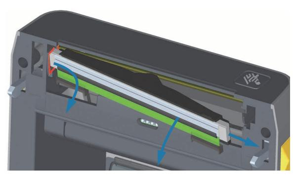
**4.** Gently but firmly pull the two printhead cable bundle connectors off of the printhead. Pull the ground wire off the printhead.
