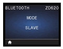
**Description:** View the Bluetooth connection pair printer's device type—Slave (typical) or Master.
