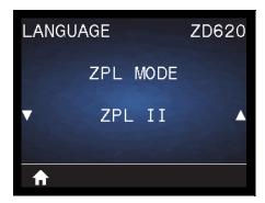
**Description:** Select the mode that matches what is used in your label formats. This printer accepts label formats written in either ZPL or ZPL II, eliminating the need to rewrite any ZPL formats that already exist. The printer remains in the selected mode until it is changed in one of the ways listed here.
