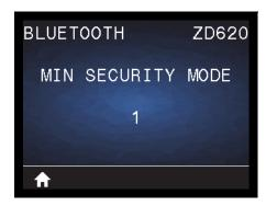
**Description:** View the printer's Bluetooth minimum level of applied security.
