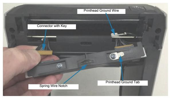
**4.** Insert the left side of the printhead assembly into the recessed slot (highlighted in red) on the left side of the printer.
