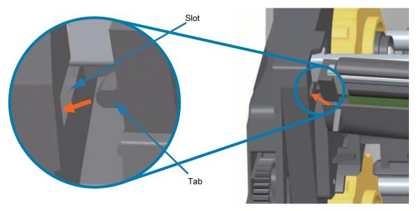
**5.** Push the right side of the printhead into the printer until the latch locks the right side of the printhead into the printer.
