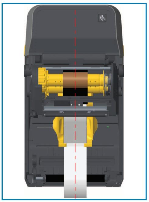
**5.** Attach the ribbon to the take up core. Use thin strip of tape to secure the ribbon to the take-up core, if your media does not have an adhesive strip on the ribbon leader like genuine Zebra<sup>@</sup> ribbon. Align the ribbon so that it will be taken straight onto the core.
