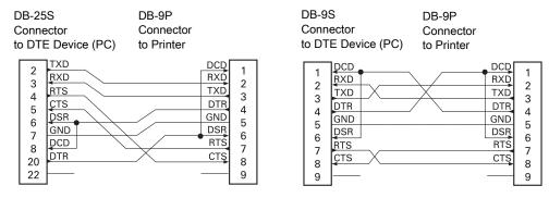
**Interconnecting to DTE Devices** — The printer is configured as data terminal equipment (DTE). To connect the printer to other DTE devices (such as the serial port of a personal computer), use an RS-232 null modem (crossover) cable.
