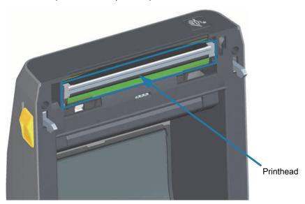
2. Push the printhead release latch away from the printhead. The right side of printhead releases.
