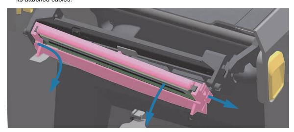
**5.** Gently but firmly pull the two printhead cable bundle connectors off of the printhead.
