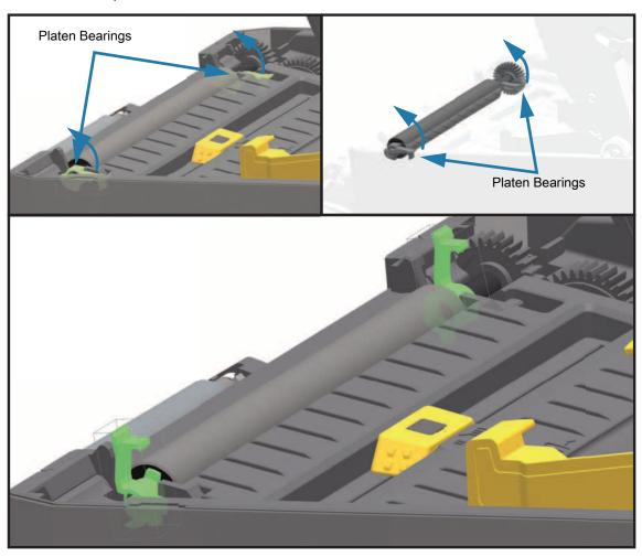
**3.** Lift the platen out of the printer's bottom frame.
