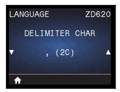
**Description:** This menu item is used to separate command parameters (command delimiter). The default prefix is the comma (,). The printer looks for this character to separate parts of ZPL/ZPL II commands. Set the delimiter character to match what is used in your label formats.
