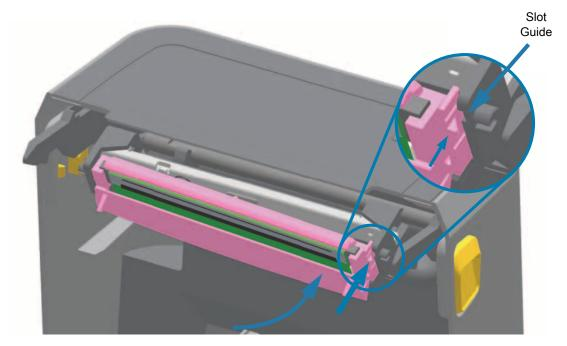
**6.** Verify that the printhead moves freely into the printer when pressure is applied (see arrow) and remains locked when pressure is released.
