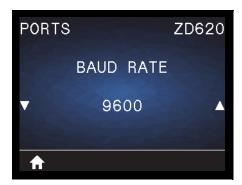
**Description:** Select the baud value that matches the one being used by the host computer.
