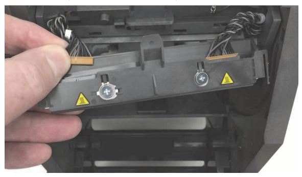
3. Insert the center tab on the printhead assembly into the center slot on the Printhead Actuator Arm.
