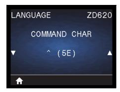
**Description:** This menu item is used to change the format command prefix. The format command prefix is an ASCII (two-digit hexadecimal value shown in parenthesis) used as a parameter place marker in ZPL/ZPL II format instructions. The printer looks for this command character to indicate the start of a ZPL/ZPL II format instruction.
