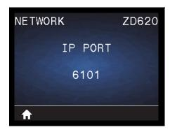
**Description:** This printer setting refers to the internal wired print servers port number that the TCP print service is listening on. Normal TCP communications from the host should be directed to this port.
