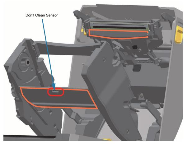
3. Release the Printhead Actuator Arm and then push the Ribbon Drive Transport into the Printhead Actuator Arm. The Release Arms will snap into place relinking the Ribbon Drive Transport to the top cover and the Printhead Actuator Arm.
