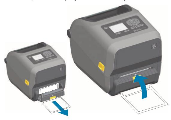
**5.** Press and release the FEED (Advance) button one or more times until a label gets presented for removal.
