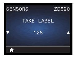
**Description:** Set the intensity of the label taken sensor circuit.
