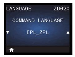
**Description:** The setting allows you to control the primary programming language variations available, such as, EPL\_ZPL, EPL (legacy language), and Hybrid\_XML\_ZPL (used for format/form variable fill-in with XML structured elements).
