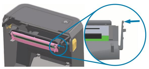
**4.** Swing the loose right side of the printhead out of the printer. Pull it to the right a little to get the left side of the printhead clear. Pull the printhead down and free of the Printhead Actuator Arm to gain access to its attached cables.
