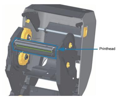
**2.** Push the printhead release latch toward the printhead (shown as green for visibility). The right side printhead releases down and away from the Printhead Actuator Arm.
