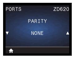
**Description:** Select the parity value that matches the one being used by the host computer.
