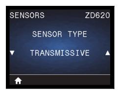
**Description:** Select the media sensor that is appropriate for the media that you are using. The reflective sensor typically is used only for black mark media. The transmissive sensor typically is used for other media types.
