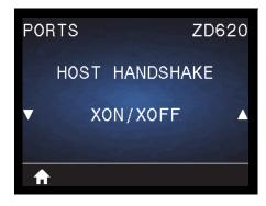
**Description:** Select the handshake protocol that matches the one being used by the host computer.
