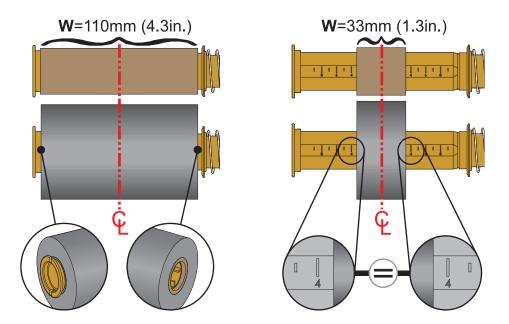
3. Place the adapter with an empty core on the take-up spindles and the adapter with the ribbon roll on the lower supply spindles. The right side of the core adapter fits on the cone tip on each of the spring loaded right side spindles. Continue pushing the adapter onto right side spindle and swing the adapter onto the left side spindle hubs. Rotate the adapters and hubs until the until notches on the adapters flange align and lock ton the left spindles hub spokes.
