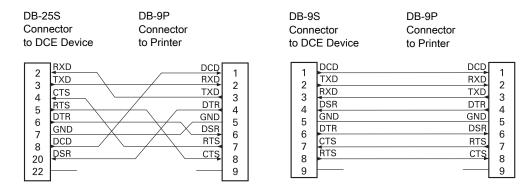
**Interconnecting to DCE Devices** — When the printer is connected via its RS-232 interface to data communication equipment (DCE) such as a modem, a STANDARD RS-232 (straight-through) interface cable must be used.
