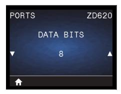
**Description:** Select the data bits value that matches the one being used by the host computer.
