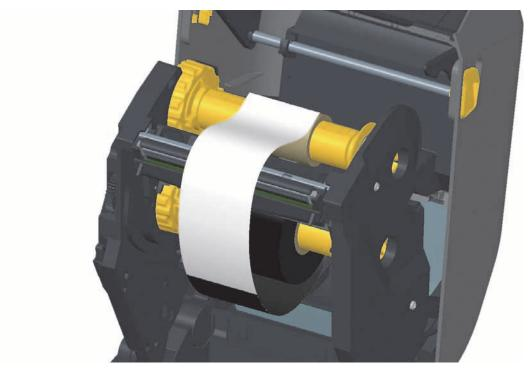
**6.** Turn the ribbon take-up hub with the top moving toward rear to remove slack from the ribbon. Rotating the hub helps to finish aligning the take up ribbon position with the supply ribbon roll. The ribbon should be wound, at minimum, one and a half times around the take-up ribbon core.
