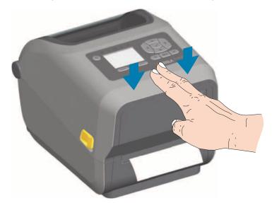
You may need a calibrate your printer for the media. The printer's sensors need to adjust to sense the label, the liner, and the distance between labels to operate properly. When reloading the same media (size, vendor, and batch), you can just press the FEED (Advance) button once to prepare the media for printing.
