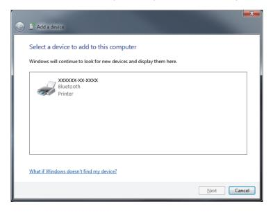
**6.** The printer will print a pairing code. Verify that the pairing numbers match with those on your display screen. If the numbers match, then press the 'Next button' in the 'Add a device' window.
