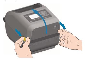
2. Open the media roll holders. Orient the media roll so that its printing surface will face up as it passes over the platen (drive) roller. Pull the media guides open with your free hand and place the media roll on the roll holders and release the guides. Verify the roll turns freely. The roll must not sit in the bottom of the media compartment.
