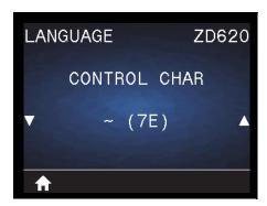
**Description:** This menu item is used to change the control command prefix. The default prefix is the tilde (~). The printer looks for this character to indicate the start of a ZPL/ZPL II command. Set the format prefix character to match what is used in your label formats.
