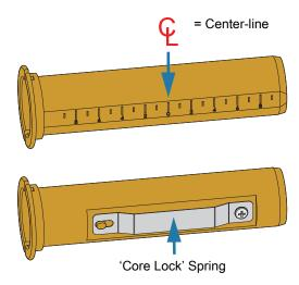
1. Load an empty ribbon core onto a ribbon core adapter. The empty ribbon core should be the same width (or larger) than the ribbon roll. Roughly center the core over the adapters center line. An empty Zebra ribbon core may be used instead of the adapter and empty non-Zebra ribbon core. One 300m empty ribbon core is supplied with the printer.
