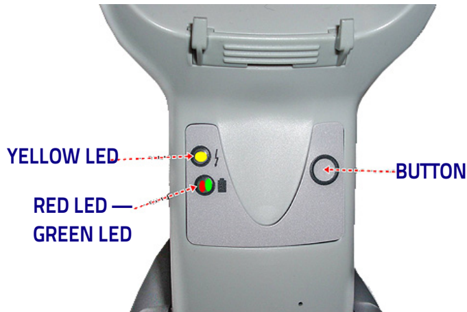
Figure 10. Gryphon Base LEDs
