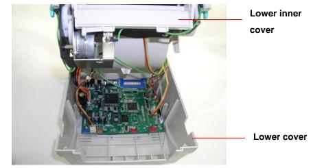
Thread the harness red connector through the cable hole at the front side of lower inner cover. Plug the red peel off module harness connector at the location JP17 (TDP-245) / JP19 (TDP-245 Plus/TDP-247/TDP-345) on the main board. Place lower inner cover to the lower cover. Install the peel-off module to the lower inner cover slot.
