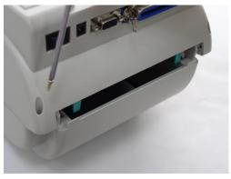
6. Remove the screw that fixes the memory card cover.
