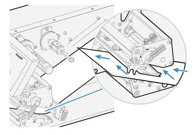
11. Pull out approximately 40 cm (15 in) of labels and remove the labels from the liner.
