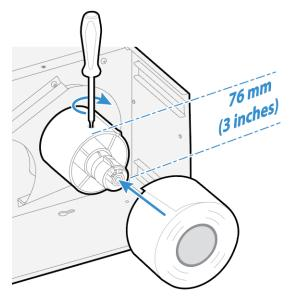
8. Fit a new roll of media onto the media supply hub and push the roll in as far as it will go.
