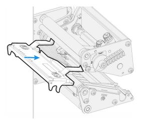
11. Turn the printhead lift lever clockwise so the magnet engages the printhead bracket.
