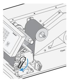
8. Press the cardboard core at the front end of the ribbon onto the rewind hub. During printing, the rewind hub rotates counter-clockwise.
