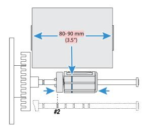
• If your ribbon is 110 mm (4.3 in) wide, compress the ribbon supply bobbin and move it so it snaps into the third (outermost) groove.
