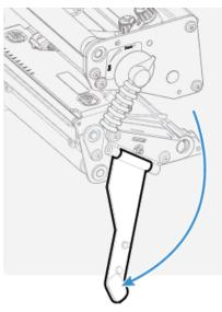
4. Turn the printhead lift lever counter-clockwise to raise the printhead.
