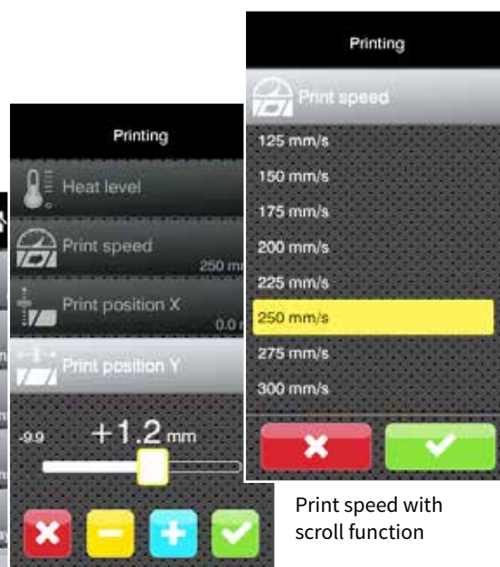
Print position Y slide control for fast adjustment ± keys for fine adjustment
