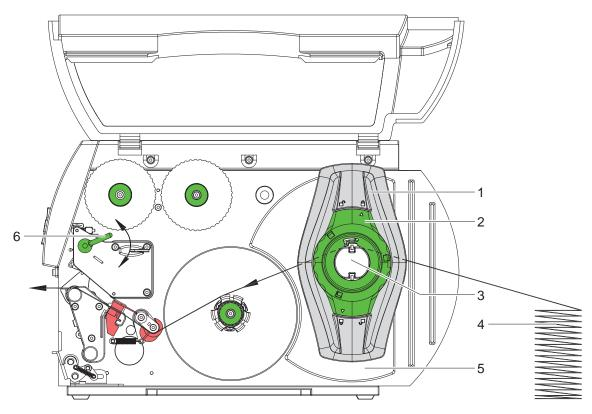
Fig. 13 Feed path of fanfold labels
