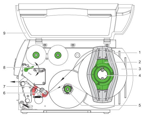
Fig. 7 Loading labels from roll
