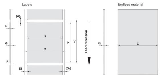
Fig. 19 Label / endless material dimensions
