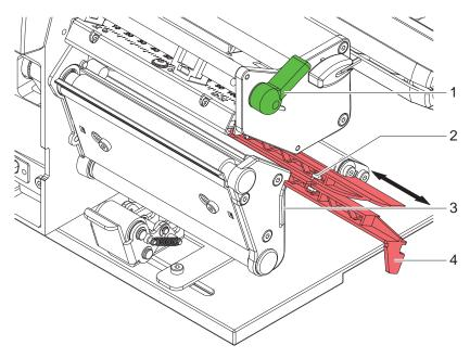
Fig. 18 Cleaning the label sensor
