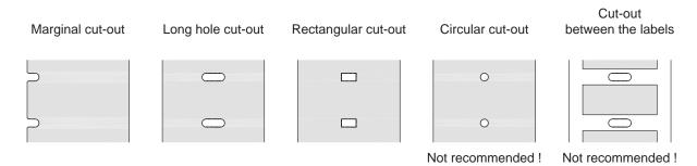
Fig. 23 Samples for cut-out marks
