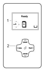
The control panel consists of a graphic display (1) and the navigator pad (2) with five integrated keys.
