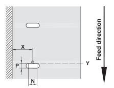
for marginal cut-out marks minimum liner thickness 0,06 mm
