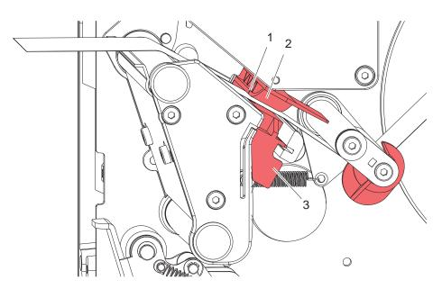
Fig. 8 Setting the label sensor
