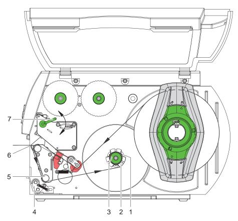
Fig. 10 Guidance of the material in peel-off mode
