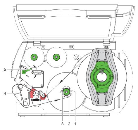
Fig. 9 Guiding the label strip in rewind mode
