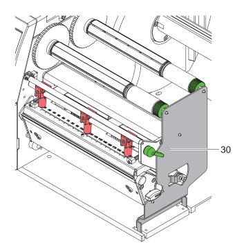
Fig. 4 Support bracket A8+
