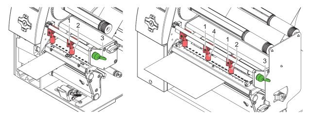
Fig. 11 Setting the head locking system
