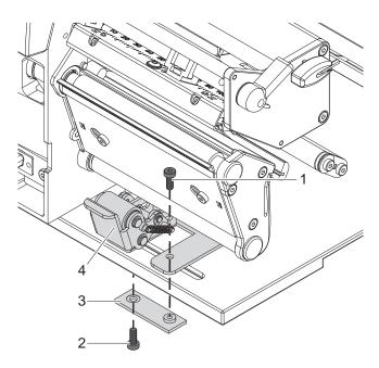
Fig. 17 Removing and installing the locking system
