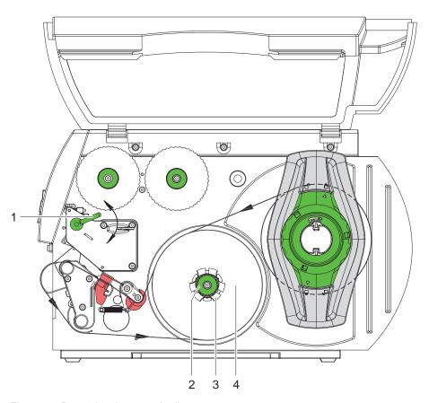
Fig. 12 Removing the wound roll
