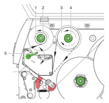
Fig. 14 Feed path of the transfer ribbon
