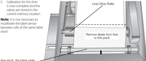
For reflective stock, the black mark — should be positioned directly under this guide roller.
