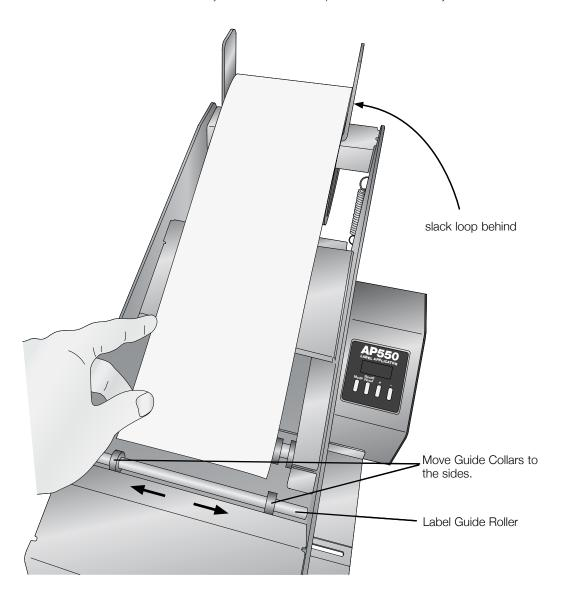
9. Use both index (pointer) fingers to roll the leading edge of the label stock UNDER the Label Guide Roller. Feed the stock forward until it enters the Sensor Housing.
