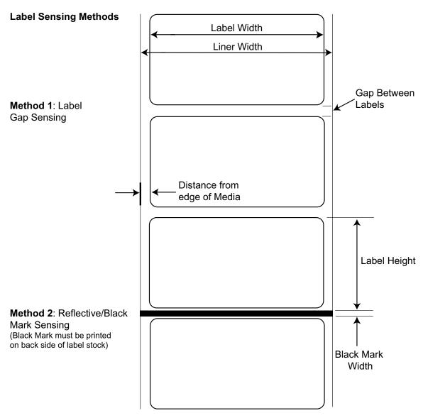
Note: See table below for Max and Min values in inches and millimeters.
